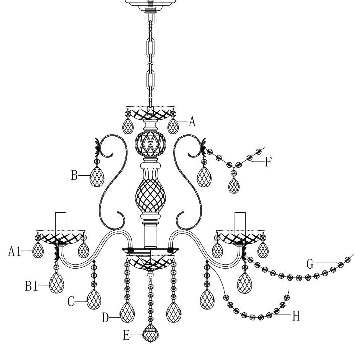
Connect both ends of F with B Connect both ends of H with C
